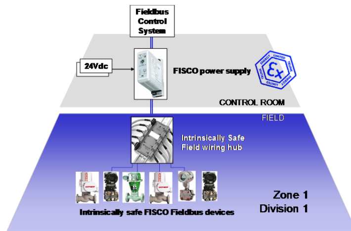
Figure 11.1: Typical FISCO segment
